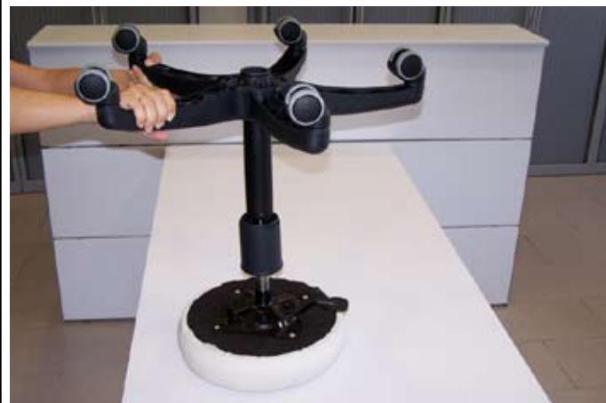
Place the 5-star base on the gas cartridge. At this time gently tap on the base as these parts are subjected to pressure.
