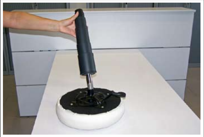
Place the gas lift cartridge in the housing plate.
